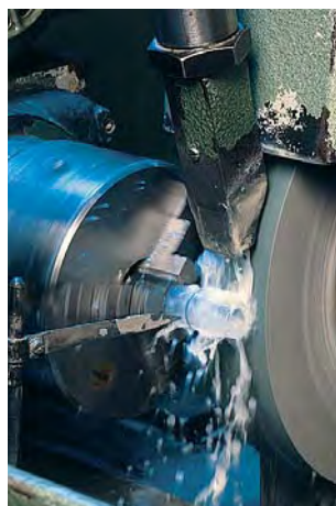
Circular grinding machines grind NS-cones half-automatically
