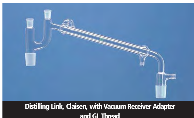
Distilling Link, Claisen, with Vacuum Receiver Adapter and Nozzle
